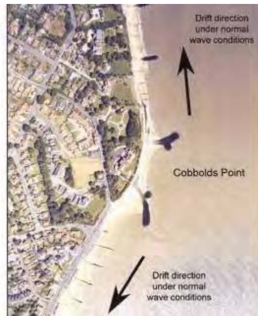
Figure 1-2 Drift parting at Cobbold's Point (Halcrow 2003)
